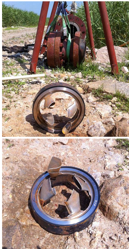
Figure 11. Bursting discs after CO 2 release from 50 mm orifice.
