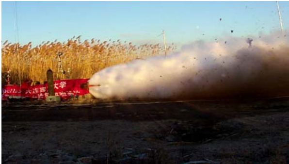
Figure 13. Initial release of the full bore rupture (233 mm i.d., release temperature 3 °C).
