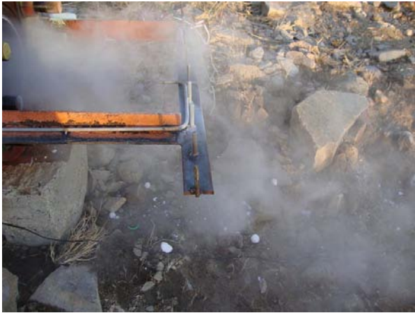
Figure 14. Near field of the full bore rupture at the end of release
