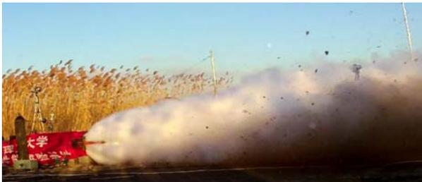
**Figure 14.** Near-field dispersion region during a full-bore rupture.
